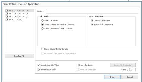
Ensure that all storeys are selected  $\Rightarrow$  Pick **Draw**  $\Rightarrow$  Click a location to insert the details. The below shows an example of a column application plan.
