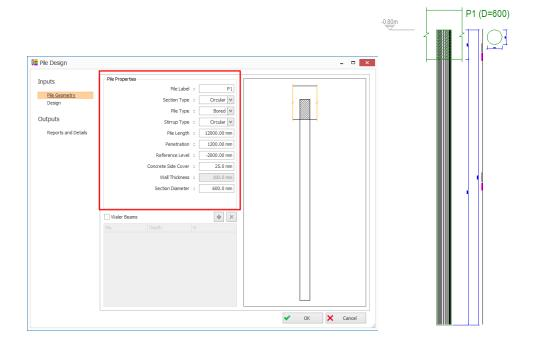
• In the **Pile Geometry** tab, input all the parameters such as Circular/ Square/ Rectangular, size, length, etc.
