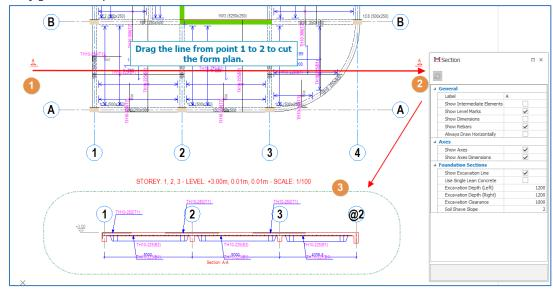
Click on the desired location to place the section detail
