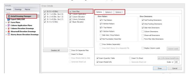
A dialog showing options to show slab reinforcement bars, member dimensions & hatching columns will be shown. Foundation plan showing raft, footing & pile caps (if any) will be shown in St:0
